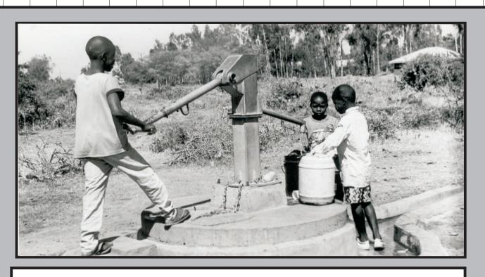
The Afridev reciprocating type hand pump has been specially designed by SKAT-HTN (Swiss Centre for Development Cooperation in Technology and Management) to meet the requirements for Village Level Operation and Maintenance (VLOM) as specified by the UNDP/World Bank. The pump has undergone extensive laboratory and field development tests and is one of only two designs which fulfils all aspects of the UNDP/World Bank specification at depths between 0 and 45m. Particular features are:
